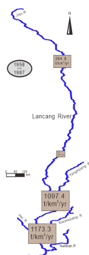
Figure 8. Sediment yield in four tracts of the Lancang catchment based on hydrological data (data from hydrological yearbook of Sanjiang catchment from 1958 to 1987 (Table S1)). River course in blue.
