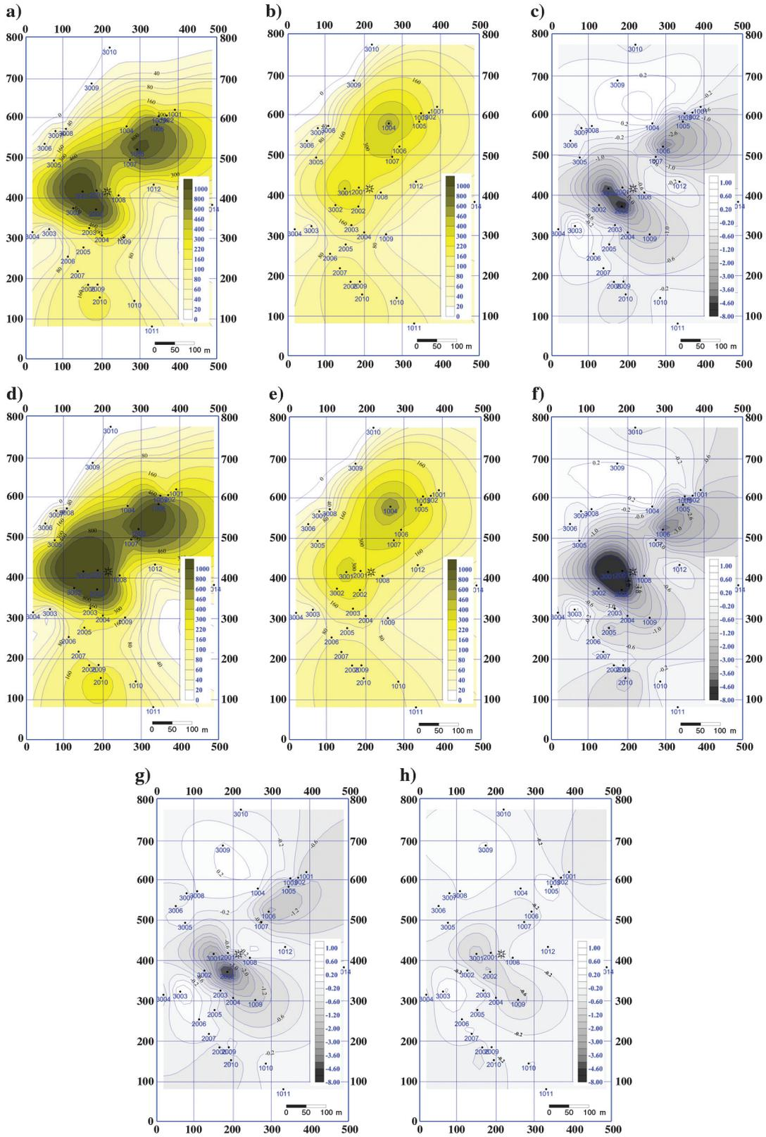
Figure 7. AMT mapping result of the test working area. (a) The prehydraulic fracturing apparent resistivity contour map at frequency 32.5 Hz; (b) is the posthydraulic fracturing apparent resistivity contour map; (c) is the variation ( $\delta = 1 - \frac{\rho_{pre}}{\rho_{post}}$ ) imaging pre- and posthydraulic fracturing; (d-f) show a corresponding result of 22.5 Hz; (g and h) show a variation of 65 and 168.7 Hz
