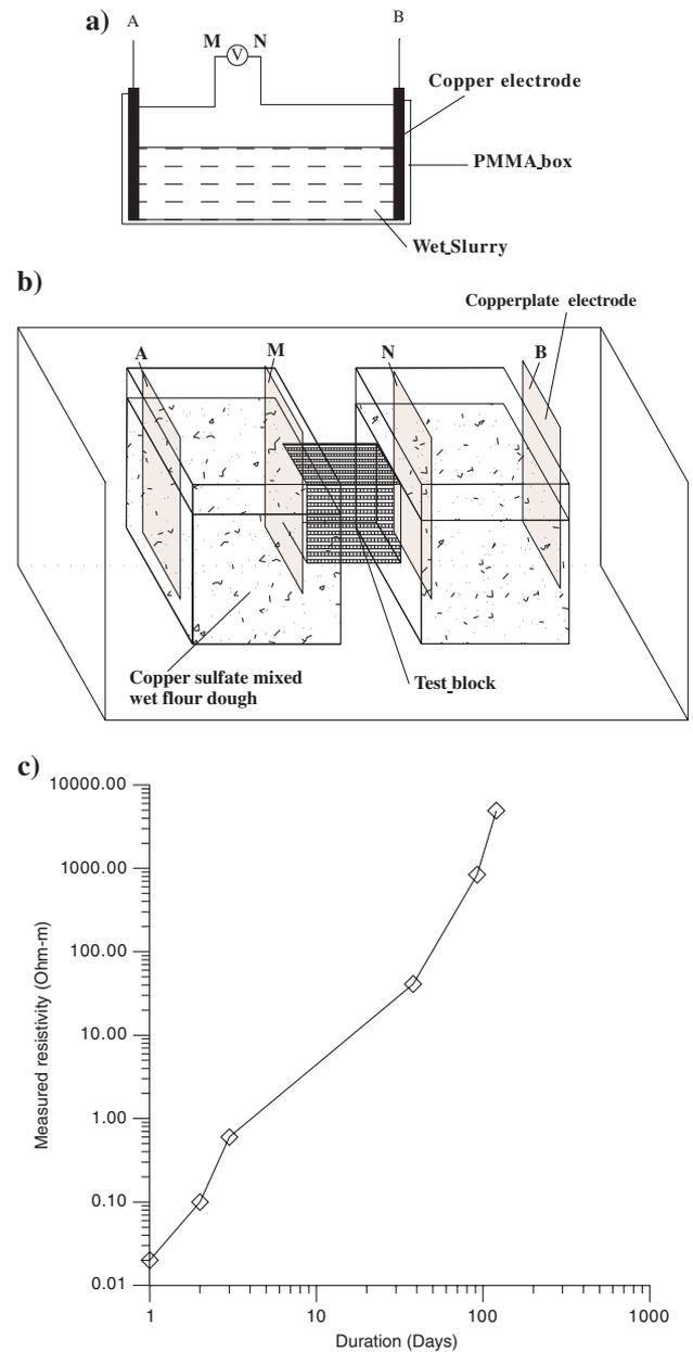
Figure 2. Laboratory resistivity measurement of the test block. (a and b) The sketch map for measuring the resistivity of wet and solidified slurry, and (c) is the measured result.
