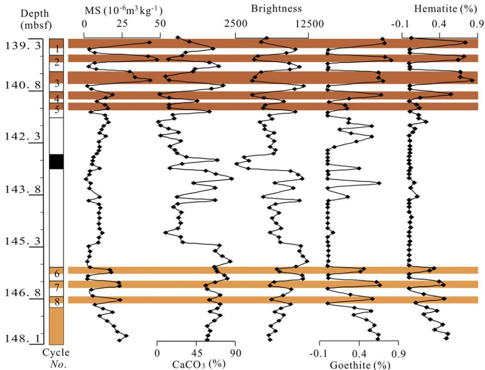
Fig. 5. Comparison of magnetic susceptibility, carbonate content, brightness, goethite content, and hematite content for Core 12X from ODP Hole 1049C (carbonate content data from Han et al., 2008).
