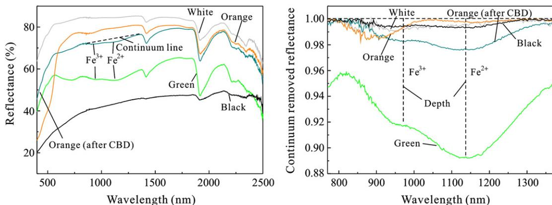
**Fig. 8.** Diffuse reflectance spectra (left) and continuum-removed reflectance spectra (right) of samples colored black, green, white, and orange. Also shown for comparison is a CBD-treated orange sample. The continuum-removal approach involved fitting a straight line to the reflectance continuum using two continuum tie points, on either side of the absorption feature ([Clark and Roush, 1984](#)).
