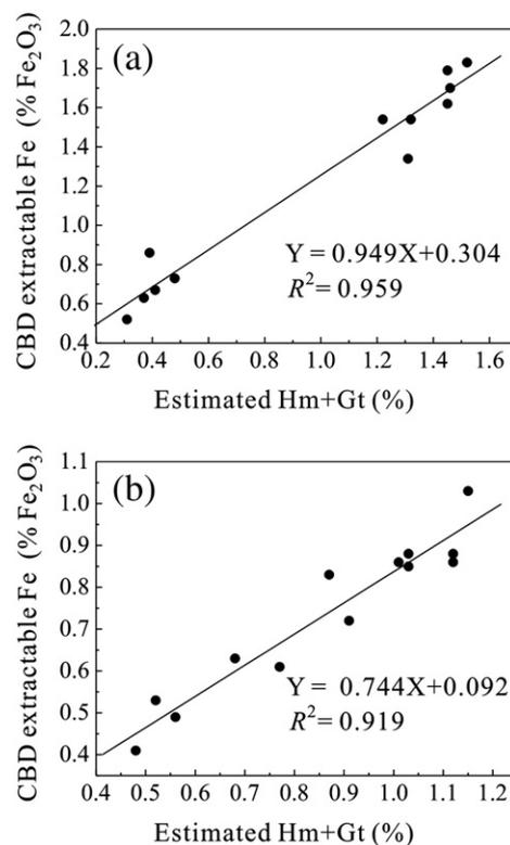
**Fig. 7.** Combined hematite–goethite concentration versus concentration of CBD extractable iron: (a) for Albian brown samples; (b) for Aptian orange samples.
