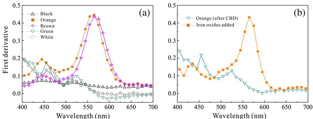
**Fig. 3.** First derivative spectral patterns for samples from Core 12X in ODP Hole 1049C. (a) First derivative spectral patterns for black, orange, brown, green, and white samples. (b) First derivative spectral patterns for an orange sample treated using the CBD procedure and subsequently iron oxides added.
