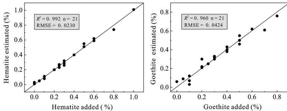
**Fig. 6.** Comparison of added, known iron oxide contents in the calibration sample set with that estimated by the regression equations. Also showing are the  $Y=X$  regression line, the square of the correlation coefficient ( $R^2$ ), and the root mean square error (RMSE).
