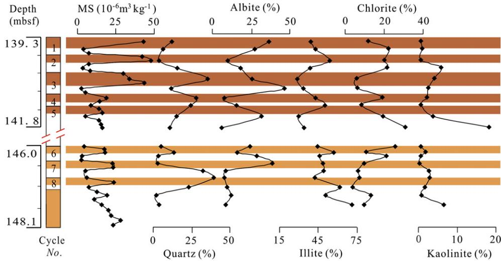
Fig. 4. Comparison of magnetic susceptibility with concentrations of quartz, albite, illite, chlorite, and kaolinite in non-carbonate fraction quantitatively analyzed by Whole Pattern Fitting using software Topas. MS: magnetic susceptibility (data from Han et al., 2008).
